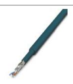
CAT5-SF/UTP cable (J-02YS(ST)C HP 2 x 2 x 24 AWG), heavy-duty installation cable, 2 x 2 x 0.22 mm $^2$ , solid conductor, shielded, outer sheath: 7.8 mm diameter, inner sheath: 5.75 mm  $\pm$  0.15 mm diameter
