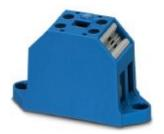
Device terminal block, nom. voltage: 1000 V, nominal current: 57 A, connection method: Screw connection, number of connections: 4, number of positions: 1, cross section: 0.5 mm² - 16 mm², AWG: 20 - 6, width: 71.3 mm, height: 40 mm, color: blue, mounting type: direct screw connection
