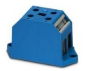
Device terminal block, nom. voltage: 630 V, nominal current: 150 A, connection method: Screw connection, number of connections: 4, cross section: 0.75 mm² - 50 mm², AWG: 18 - 1/0, width: 34.75 mm, height: 44.9 mm, color: blue, mounting type: direct screw connection
