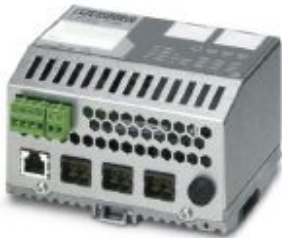
Ethernet Switch, one port in RJ45 format and three ports in POF SC-RJ format for PROFINET RT/IRT, DIN rail mountable
