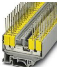
Feed-through terminal block, connection method: Slip-on connection, cross section: 0.5 mm 2 - 6 mm 2 , AWG: 20 - 10, width: 6.2 mm, color: gray, mounting: NS 35/7,5, NS 35/15, NS 32
