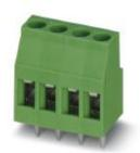
PCB terminal block, nominal current: 24 A, rated voltage (III/2): 400 V, nominal cross section: 2.5 mm², pitch: 5 mm, number of positions: 8, connection method: Screw connection with tension sleeve, mounting: Wave soldering, conductor/PCB connection direction: 0 °, color: green, Pin layout: Linear pinning, Solder pin [P]: 3.6 mm. The article can be aligned to create different nos. of positions!
