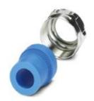
Half screw connection Pg21, made of metal, consisting of rubber seal with one hole and one pressure screw, for type 2 - 4 housings, cable [mm] 14 - 18
