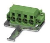
PCB connector, nominal current: 76 A, rated voltage (III/2): 1000 V, nominal cross section: 16 mm², number of positions: 4, pitch: 10.16 mm, connection method: Push-in spring connection, color: green, contact surface: Silver
