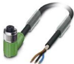
Sensor/actuator cable, 3-position, PUR halogen-free, black-gray RAL 7021, shielded, free cable end, on Socket angled M12, coding: A, cable length: 5 m
