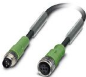
Sensor/actuator cable, 3-position, PUR halogen-free, black-gray RAL 7021, Plug straight M8, on Socket straight M12, coding: A, cable length: 1.5 m
