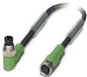
Sensor/actuator cable, 4-position, PUR halogen-free, black-gray RAL 7021, Plug angled M8, on Socket straight M8, cable length: 0.6 m
