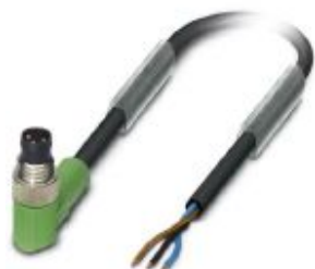
Sensor/actuator cable, 3-position, PUR halogen-free, black-gray RAL 7021, Plug angled M8, on free cable end, cable length: 5 m
