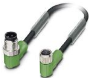
Sensor/actuator cable, 3-position, PUR halogen-free, black-gray RAL 7021, Plug angled M12, coding: A, on Socket angled M8, cable length: 1.5 m
