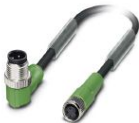
Sensor/actuator cable, 3-position, PUR halogen-free, black-gray RAL 7021, Plug angled M12, coding: A, on Socket straight M8, cable length: 0.3 m
