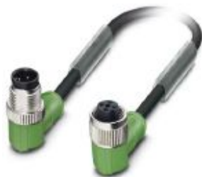
Sensor/actuator cable, 4-position, PUR halogen-free, black-gray RAL 7021, Plug angled M12, coding: A, on Socket angled M12, coding: A, cable length: 3 m
