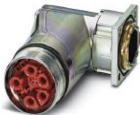
Device connector for front wall, SB, angled rotatable, shielded: yes, for standard and SPEEDCON interlock, M40, type of contact: Socket, Crimp connection, Axial O-ring, 4x Ø4,2
