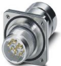
Rear panel feed-through, straight, Screw locking, M23, number of positions: 5+PE, type of contact: Pin, Axial O-ring, 4xM3, shielded: yes, cable diameter range: 11 mm ... 14 mm, number of positions: 6, connection method: Crimp connection
