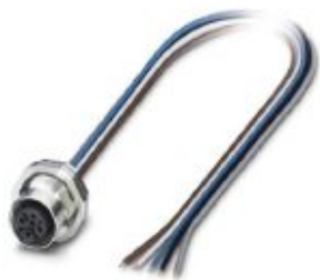
Sensor/actuator flush-type socket, 5-pos., M12, A-coded, rear/screw mounting with Pg9 thread, with 0.5 m TPE litz wire, 5 x 0.34 mm 2 , stainless steel version
