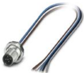
Sensor/actuator flush-type plug, 5-pos., M12, A-coded, rear/screw mounting with Pg9 thread, with 0.5 m TPE litz wire, 5 x 0.34 mm 2 , stainless steel version
