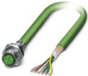
Bus system flush-type female connector, INTERBUS, 5-pos., M12, shielded, B-coded, rear/screw mounting with M16 thread, with 0.5 m bus line
