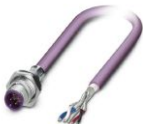
Bus system flush-type plug, DeviceNet/CANopen, 5-pos., M12, shielded, A-coded, rear/screw mounting with M16 thread, with 5 m bus cable, 2 x 0.2 mm 2 , 2 x 0.32 mm 2
