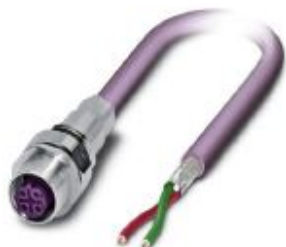
Bus system flush-type socket, PROFIBUS, 2-pos., M12, shielded, B-coded, front/screw mounting with M16 thread, with 1 m bus cable, 2 x 0.25 mm 2
