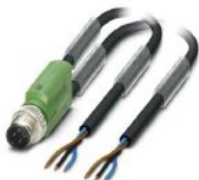
Sensor/actuator cable, 3-position, PUR halogen-free, black-gray RAL 7021, Plug straight M12 SPEEDCON, coding: A, on free cable end and free cable end, cable length: 1.5 m
