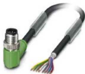
Sensor/actuator cable, 8-position, PUR halogen-free, black-gray RAL 7021, shielded, Plug angled M12, coding: A, on free cable end, cable length: 5 m
