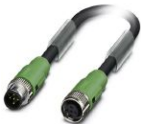
Sensor/actuator cable, 5-position, PUR, black-gray RAL 7021, Plug straight M12 SPEEDCON, coding: A, on Socket straight M12 SPEEDCON, coding: A, cable length: 0.13 m
