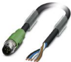
Sensor/actuator cable, 5-position, PUR, black-gray RAL 7021, Plug straight M12 SPEEDCON, coding: A, on free cable end, cable length: 5 m
