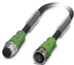
Sensor/actuator cable, 4-position, PUR, black-gray RAL 7021, Plug straight M12, coding: A, on Socket straight M12, coding: A, cable length: 0.5 m
