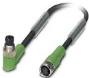
Sensor/actuator cable, 3-position, PUR halogen-free, black-gray RAL 7021, Plug angled M8, on Socket straight M8, cable length: 1.5 m
