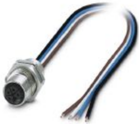
Flush-type connector, Power, 4-position, Socket, M12, L - Power, Rear mounting, M16 x 1.5, Individual wires, cable length: 0.2 m, 1.31 mm 2 , UL/cUL stranded hook-up wire
