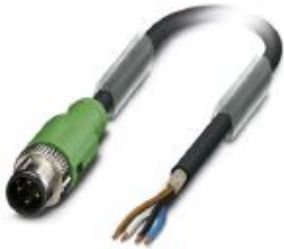
Sensor/actuator cable, 4-position, PUR halogen-free, black-gray RAL 7021, shielded, Plug straight M12 SPEEDCON, coding: A, on free cable end, cable length: 0.7 m
