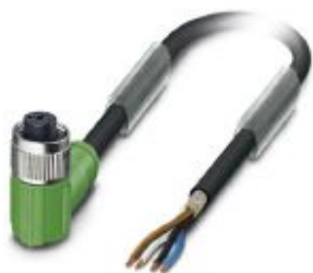
Sensor/actuator cable, 4-position, PVC, gray RAL 7001, shielded, free cable end, on Socket angled M12, coding: A, cable length: 45 m
