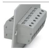
Panel feed-through terminal block, connection method: Screw connection with tension sleeve, Screw connection with tension sleeve, number of positions: 1, load current: 76 A, cross section: 0.5 mm² - 25 mm², connection direction of the conductor to plug-in direction: 0 °, width: 12.1 mm, color: gray
