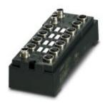
The local bus device has digital inputs and outputs. Functions: 8 digital inputs, 3 ms filter time, 8 digital outputs of 500 mA each, 500 kbaud/2 Mbaud selection, channel-specific diagnostics, short-circuit and overload protection, M12 fast connection technology.
