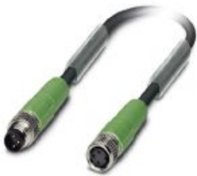
Sensor/actuator cable, 3-position, PUR halogen-free, black-gray RAL 7021, shielded, Plug straight M8, on Socket straight M8, cable length: 0.6 m
