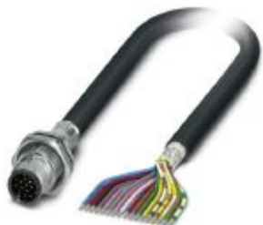
Flush-type plug, shielded, 17-pos., M12, A-coded, rear/screw mounting with M16 thread, with 1 m cable, 17 x 0.14 mm 2
