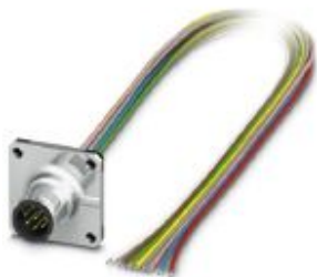
Sensor/Actuator flush-type plug, 8-pos., M12, A-coded, front/square flange mounting, with 0.5 m TPE litz wire, 8 x 0.25 mm 2
