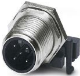
Sensor/actuator flush-type connector, connector, 5-pos., M12, shielded, A-coded, rear/screw mounting with M12 thread, with polarity protection, with angled solder connection
