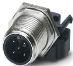
Sensor/actuator flush-type plug, 5-pos., M12, shielded, A-coded, rear/screw mounting with M12 thread, with polarity protection, with straight solder connection
