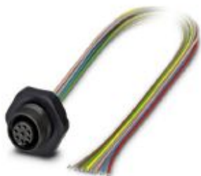
Sensor/Actuator flush-type connector, socket, 8-pos., M12, A-coded, rear/screw mounting with Pg9 thread, with 0.5 m TPE litz wire, 8 x 0.25 mm 2 , plastic version
