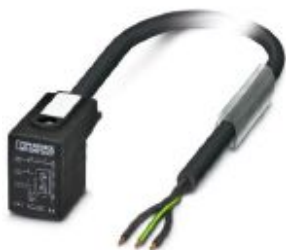
Sensor/actuator cable, 3-position, PUR halogen-free, black-gray RAL 7021, free cable end, on Valve connector BI (11 mm), with 1 LED, connected with Z diode, cable length: 10 m
