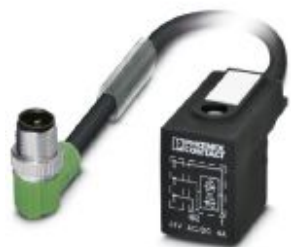
Sensor/actuator cable, 3-position, PUR halogen-free, black-gray RAL 7021, Plug angled M12 SPEEDCON, coding: A, on Valve connector BI (11 mm), with 1 LED, connected with Z diode, cable length: 0.6 m
