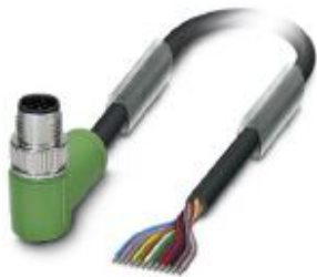
Sensor/actuator cable, 12-position, PUR halogen-free, black RAL 9005, Plug angled M12 SPEEDCON, coding: A, on free cable end, cable length: 1.5 m
