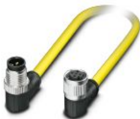
Sensor/actuator cable, 5-position, PVC, yellow, Plug angled M12, coding: A, on Socket angled M12, coding: A, cable length: 3 m
