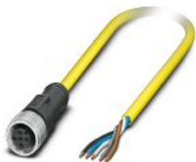
Sensor/actuator cable, 5-position, PVC, yellow, free cable end, on Socket straight M12, coding: A, cable length: 10 m
