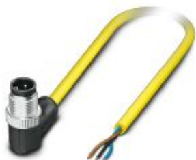
Sensor/actuator cable, 3-position, PVC, yellow, Plug angled M12, coding: A, on free cable end, cable length: 10 m
