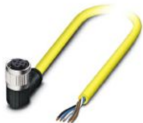
Sensor/actuator cable, 5-position, PVC, yellow, free cable end, on Socket angled M12, coding: A, cable length: 5 m
