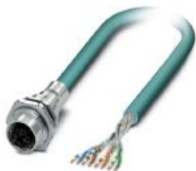
Assembled Ethernet cable, CAT6 A , shielded, 4-pair, 26 AWG stranded (7-wire), RAL 5021 (water blue), M12 flush-type socket, rear/screw mounting with M16 thread to free cable end, length: 2 m
