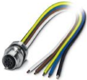
Sensor/actuator flush-type socket, 5-pos., M12, B-coded, front/screw mounting with Pg9 thread, with 0.5 m TPE litz wire, 5 x 0.34 mm 2 , stainless steel version
