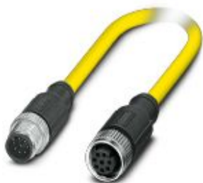
Sensor/actuator cable, 8-position, PVC, yellow, shielded, Plug straight M12, coding: A, on Socket straight M12, coding: A, cable length: 15 m
