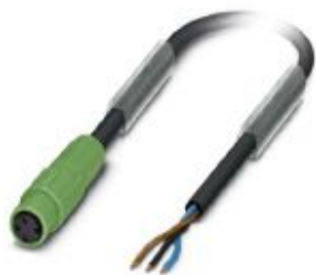
Sensor/actuator cable, 3-position, PUR halogen-free, black-gray RAL 7021, free cable end, on Socket straight M8 Snap-in, cable length: 0.6 m
